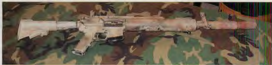
Prototype Special Purpose Rifle (SPR) with collapsible stock and suppressor mounted on an 18-inch fluted barrel: short, accurate, lightweight.
